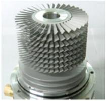
*Aluminum rotor with EDM bladed stages*
