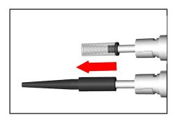
➡ Pull adapter with hose out of the VHC<sup>pro</sup>.
