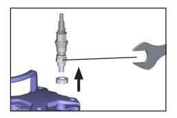
Unscrew hose nozzle, or hose nozzle with coupling, using an open-ended wrench.
