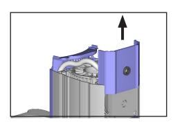
► Remove the cover of the housing cover from the housing.
