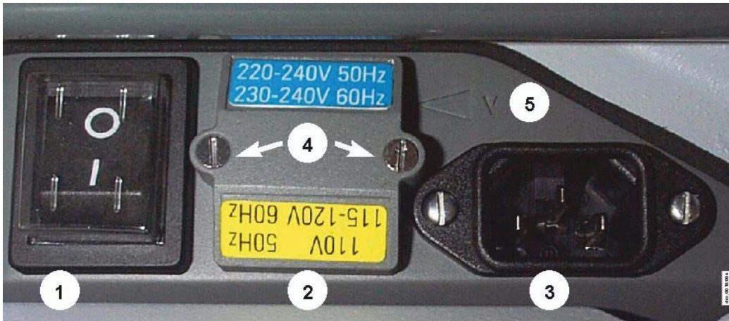
Figure 4 - Electrical interface: single-phase pumps
