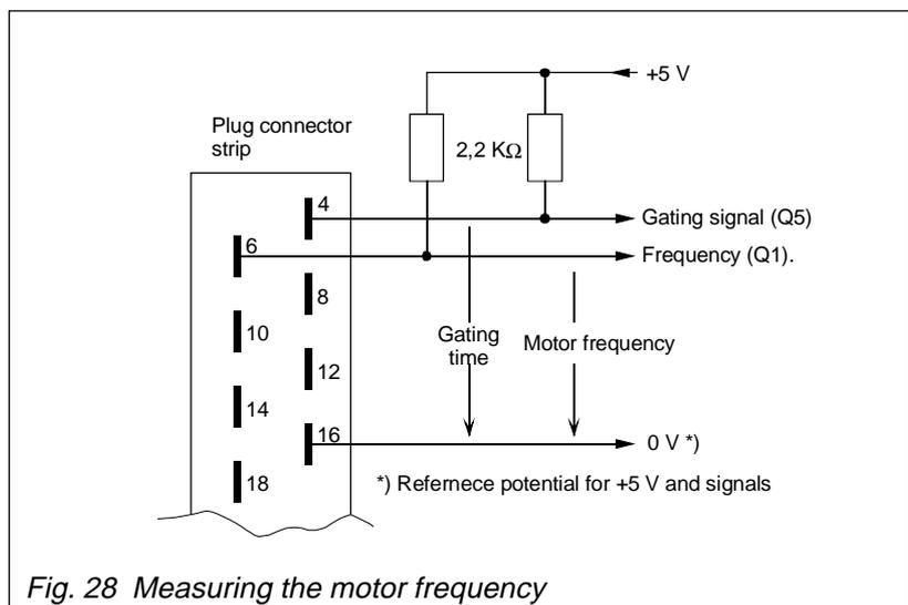
Fig. 28 Measuring the motor frequency
