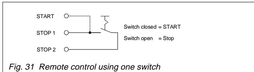
Fig. 31 Remote control using one switch
