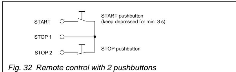
Fig. 32 Remote control with 2 pushbuttons
