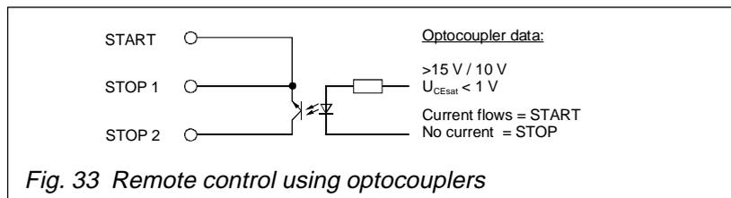
Fig. 33 Remote control using optocouplers
