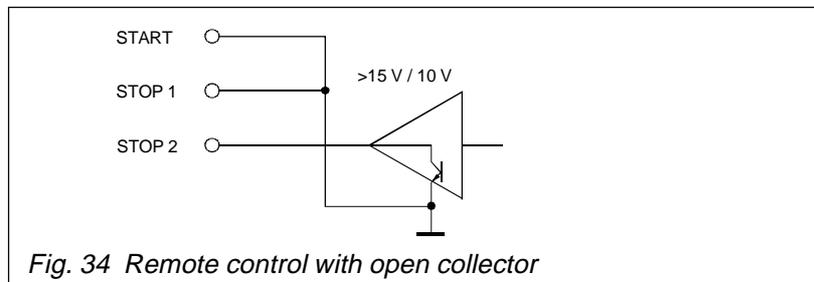
Fig. 34 Remote control with open collector
