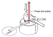
Following calibration of the zero point, the gauge returns automatically to measuring mode. The LED <RUN> lights up.
