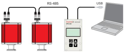
Fig. 4: Connections diagram gauge/DPG 202
