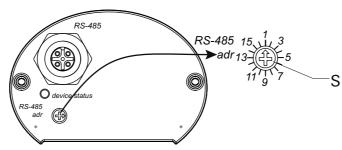
Fig. 3: Setting the address selection switch
