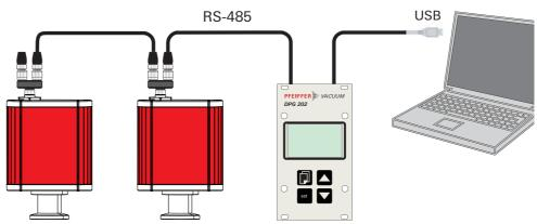
Fig. 4: Connections diagram gauge/DPG 202
