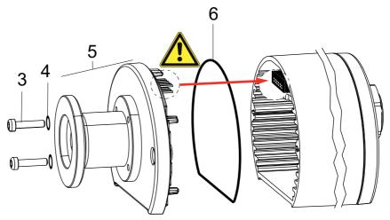
Fig. 7: Replacing the sensor assembly
