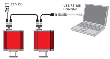
Fig. 5: Connections diagram gauge - USB/RS-485 converter
