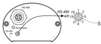
Fig. 3: Setting the address selection switch
