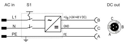
Fig. 5: Connection diagram TPS
