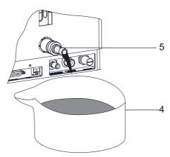
Fig. 13: Fitting of the drain connector
