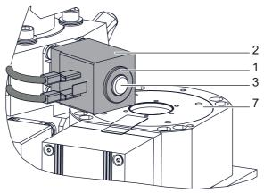
Fig. 20: Dismantling the coil
