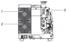
Fig. 28: Air filters location
