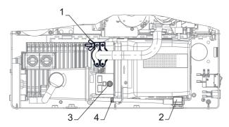
Fig. 16: Dismantling the primary pump
