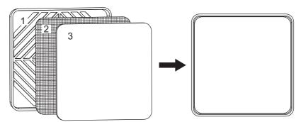
Fig. 29: Air filter assembly
