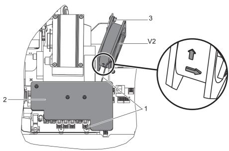
Fig. 26: Maintenance of the turbomolecular pump fan
