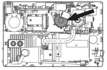
Fig. 19: Turbomolecular pump location
