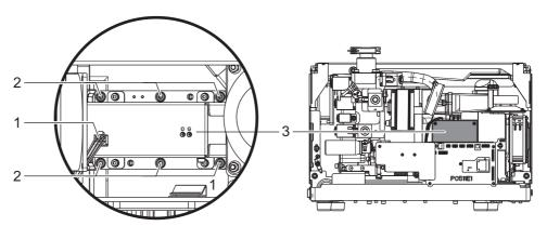
Fig. 6: Dismantling the analyzer cell
