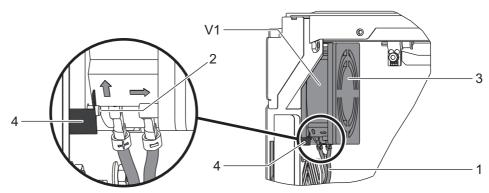
Fig. 25: Placing of fan and harness
