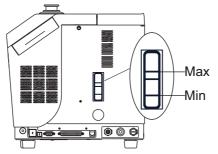
Fig. 12: Oil level check
