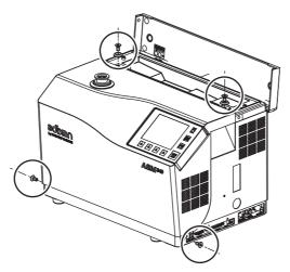
Fig. 2: Location of the front cover dismantling screw
