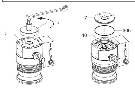
Fig. 21: Assembly / Disassembly of the operating fluid reservoir
