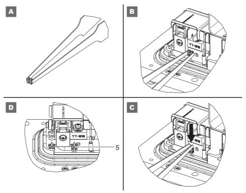
Fig. 10: Fitting of the fastening clip
