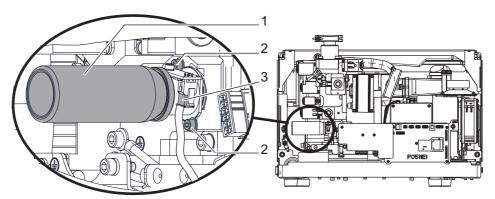
Fig. 4: Calibrated leak maintenance
