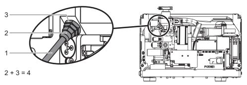
Fig. 30: Maintenance of the vacuum block air filter
