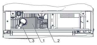
Fig. 17: Internal oil mist eliminator disassembly
