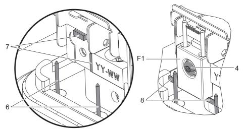
Fig. 9: Positioning the filament
