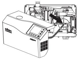
Fig. 3: Disassembly of the front cover
