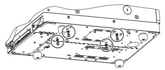
When dismantling the primary pump to send it to the service center, keep the tightening clamp, power cable and entire mist eliminator unit (mist eliminator + bracket + screws). **Never send accessories with the pump.**
