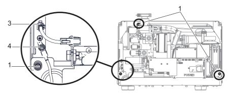
→ Before reassembling the front cover, make sure that the 5 fixing screws for the rear cover on the frame are in place and properly screwed.
