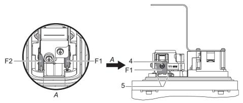
Fig. 8: Dismantling the filament
