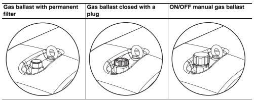
Fig. 6: The various gas ballast models
