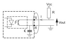
Vcc : direct voltage delivered by the installation \*(between 7 and 30 VDC) R : resistance value \*
