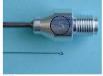
• Sniffer probe equipped with a ∅ 0.35 mm needle is marked "5".
