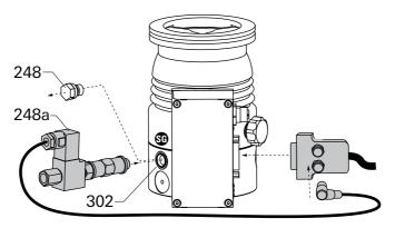
Fig. 13: Connecting the sealing gas valve
