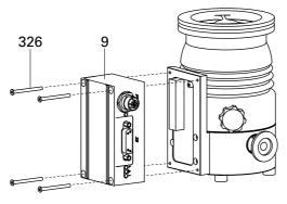
Fig. 17: Assembly / disassembly of the TC 110
