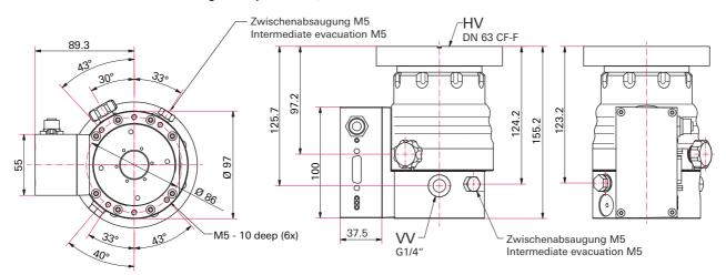
Fig. 19: SplitFlow 50, DN 63 CF-F
