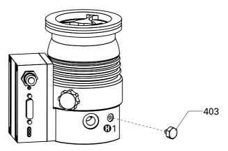
Fig. 9: Connecting the intermediate evacuation
