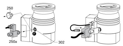
Fig. 11: Connecting the venting valve
