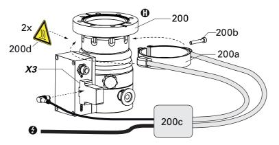
Fig. 12: Connecting the heating jacket
