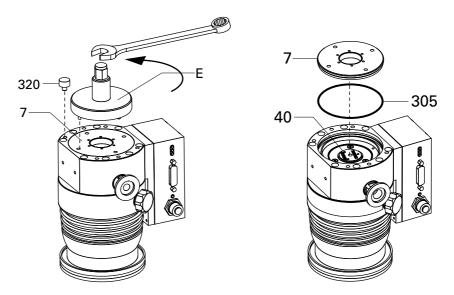
Fig. 16: Assembly / Disassembly of the operating fluid reservoir
