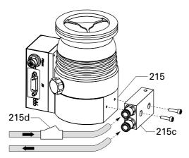
Fig. 14: Connecting the cooling water
