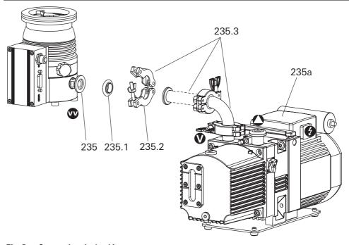
Fig. 5: Connecting the backing pump
