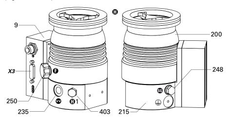
Fig. 2: View of SplitFlow 50 with TC 110
