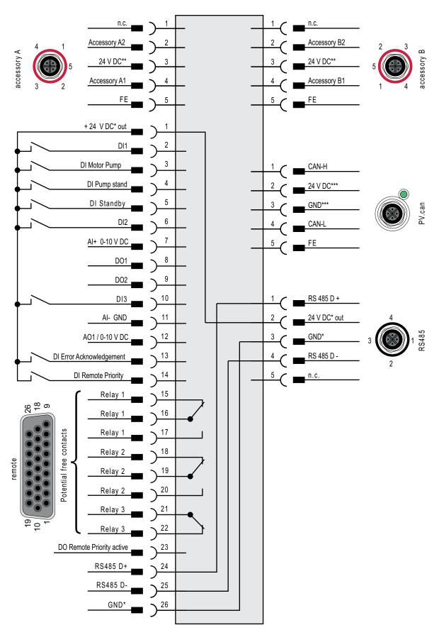
Fig. 2: Diagram and assignments of the connection panel
