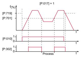
Fig. 8: Rotation speed switch points 1 & 2 active, [P:701] < [P:719]
