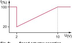
Fig. 9: Speed actuator operation
