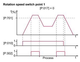
Fig. 6: Rotation speed switch point 1 active
