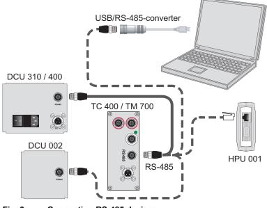
Fig. 3: Connecting RS-485 devices
