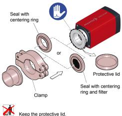
Remove the protective lid and connect the product to the vacuum system.
