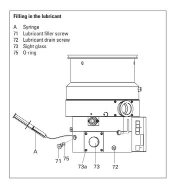
→ Screw back in lubricant filler screw 71 with 0-ring 75.
