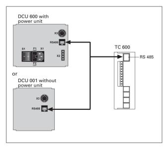
The serial interface is galvanically and safely separated from the maximum supply voltage from the TC 600.
