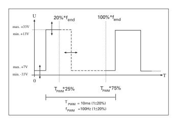
If no signal is present the pump accelerates up to its final rotation speed.
