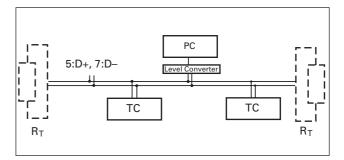
All units connected to the bus must have differing serial interface addresses (parameter 797).
