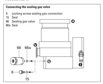
Please refer to Operating Instructions PM 800 229 BN for details on installing the sealing gas valve and adjusting the sealing gas flow.
