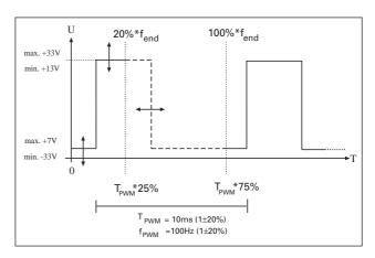
If no signal is present the pump accelerates up to its final rotation speed. A PWM adapter box for rotation speed setting operations for the turbopump is available as an option (please see "Accessories").
