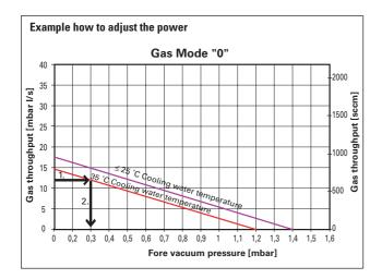
The following gas type characteristics lines enable you to adjust the power properly. At a cooling water temperature between 25  $^{\circ}$ C and 35  $^{\circ}$ C you have to draw your own gas type characteristics line.
