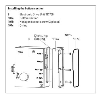
→ First pull the corresponding cables through the inserts with screwed cable glands and the cover 107d and insert the cables at the TC 750.
