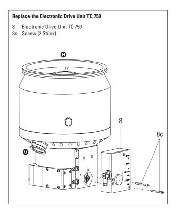
→ Assemble the new Electronic Drive Unit TC 750 on the turbopump and connect again.
