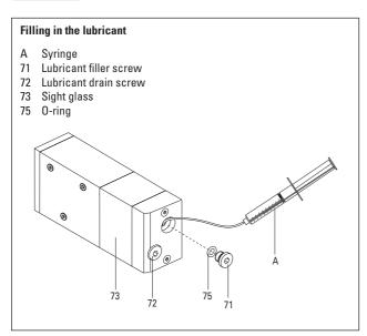
→ Screw back in lubricant filler screw 71 with the 0-ring 75.
