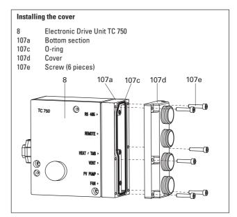
→ Firmly tighten the screwed cable glands at the cover 107d.
