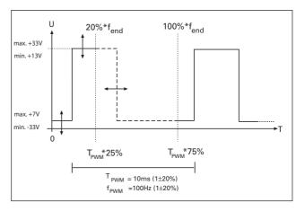
If no signal is present the pump runs up to its final rotation speed.
