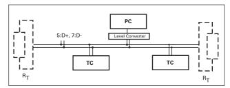
All units connected to the bus must have differing serial interface addresses (parameter 797).
