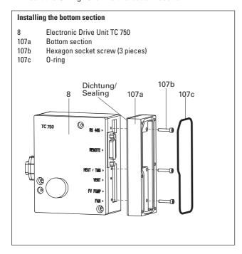
→ First pull the corresponding cables through the inserts with screwed cable glands and the cover 107d and insert the cables at the TC 750.
