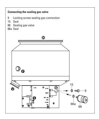
Please refer to Operating Instructions PM 0229 BN for details on installing the sealing gas valve and adjusting the sealing gas flow.
