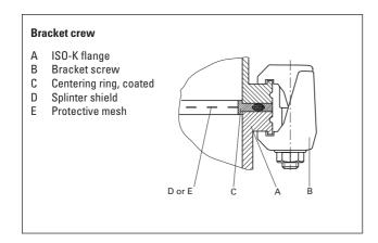
→ The clamps need to be tightened crosswise in three steps. Tightening torque: 5 Nm, 15 Nm, 25 ±2 Nm.
