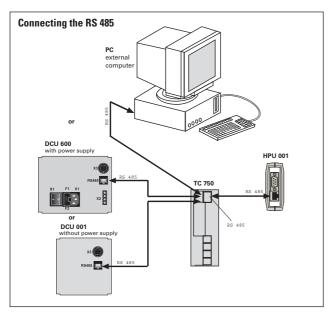
The serial interface is galvanically and safely separated from the maximum supply voltage from the TC 750.
