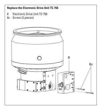
→ Assemble the new Electronic Drive Unit TC 750 (order number for the TC 750 please see Section 10. Spare Parts) on the turbopump and connect again.
