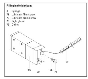
➡ Screw back in lubricant filler screw 71 with the O-ring 75.
