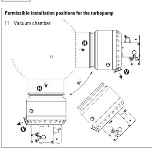
The maximum loading capacity of the high vacuum flange is 2000 N (equivalent to 200 kg). Asymmetric loading on the high vacuum flange must be avoided.
