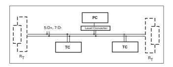
All units connected to the bus must have differing serial interface addresses (parameter 797). The group address of the TC 750 is 960.
