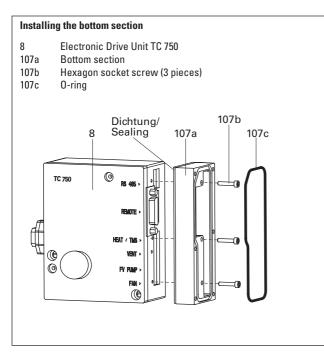
First pull the corresponding cables through the inserts with screwed cable glands and the cover 107d and insert the cables at the TC 750.
