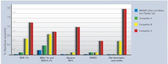
Figure 1: Residual volume in BRAND Ultra Low Retention tips, and Low Retention tips from other manufacturers in comparison with different liquids
