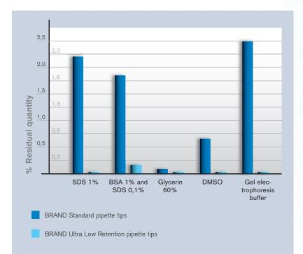
Figure 2: Residual volume in 200  $\mu I$  BRAND standard tips, BRAND Ultra Low Retention tips in comparison with different liquids
