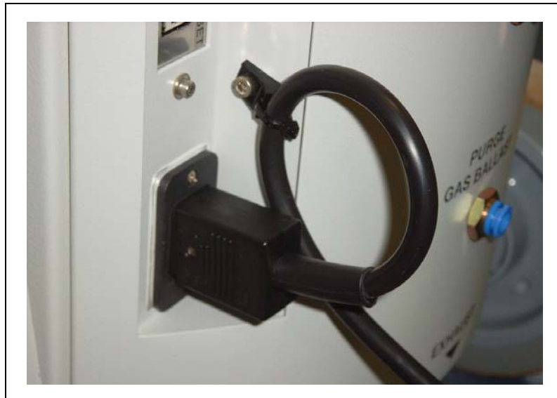
Fig. 2-4 secure fixture power cord
