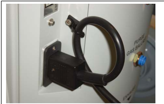
Fig. 2-4. secure fixture power cord
