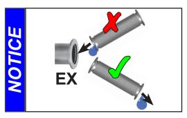
Always install outlet tubing descending from the pump to avoid backflow of condensate towards the pump.
