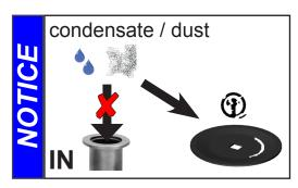
Prevent internal condensation, transfer of liquids or dust. The diaphragms and valves will be damaged, if liquids are pumped in significant amounts.
