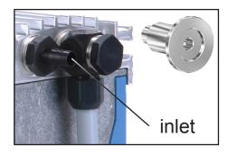
In case, install a small flange connection KF DN 16 (thread G1/8") instead, see "Accessories", pg. 44).
