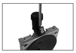
Loosen connection fastener slightly.
