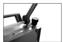
Tighten the union nut (K) of the hose connection with an open-ended wrench w/f 17.
