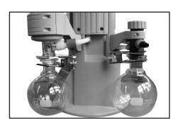
➡ Assemble catchpots (10) with joint clips.
