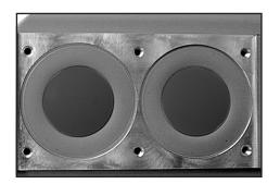
Bring the diaphragms (E) into a position, in which they are in contact with the housing (I) and centered with respect to the bore.
