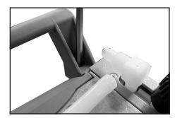
Attach the handle at the housing cover (use 5 mm wide Allen key)
