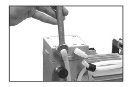
Slip the hoses onto the hose connectors by turning the fittings with an open-ended 14 mm wrench.
