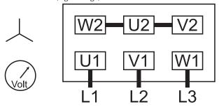
Double star connection, multi-voltage motor (low voltage):
