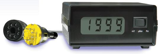
**The Model 100H** is a portable digital vacuum instrument that reads from 1 milliTorr (1 x 10<sup>-3</sup> Torr) up to 1999 millitorr/microns and comes standard with a Hastings DV-6M thermocouple vacuum gauge tube.
