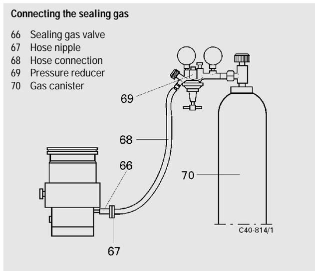
See operating instructions for the sealing gas for setting sealing gas levels.
