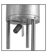
Remove the cold trap from the vacuum installation to drain the coolant if necessary.
