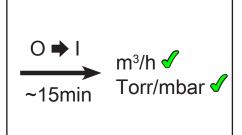
A warm up period (approximately 15 min.) is required to ensure that the rated ultimate vacuum and pumping speed are attained.
