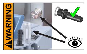
Operation with silencer at the outlet: Operating the pump at a high inlet pressure or pumping dusty gases for a long time may cause clogging of the silencer. Check the silencer regularly and replace if necessary, or install a hose nozzle with sealing ring instead (see "Accessories", pg. 51).
