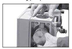
➡ By turning eccentric bushing (front of connecting rod), bring connecting rod into a position in which diaphragm is in contact with housing and centered with respect to bore.
