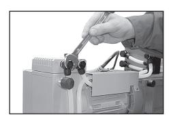
▶ Use open-ended wrench, remove screw-in fittings from all pump heads and remove manifold.
