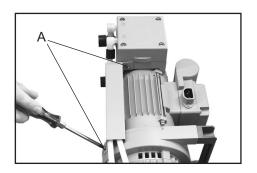
Remove the cover plate. Use a Phillips screw driver size 2 to loosen both screws (A). Pay attention to lock washers.
